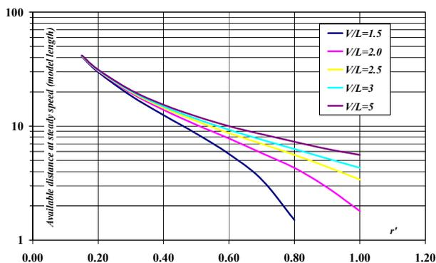
Figure 6: Influence of speed and  $r'$  on duration of stationary conditions (ship length) for a complete turn.
