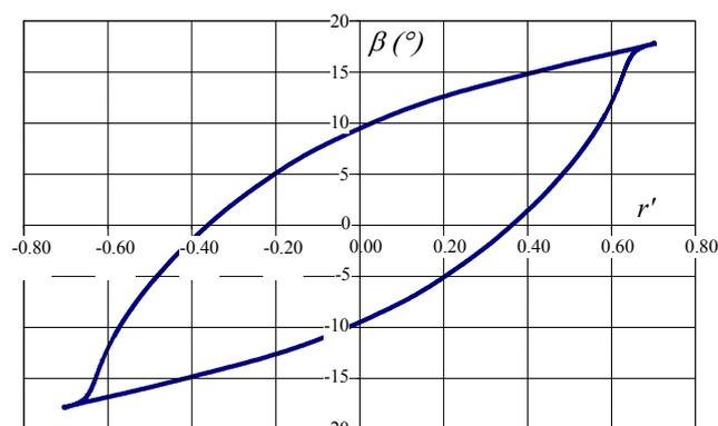
Figure 5: Yaw rate, drift angle envelope for a surface ship
